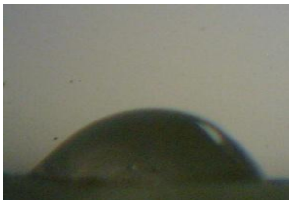
Figure: 4 Contact angle between CdTeO 3 films on the glass with water
